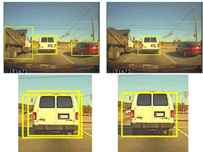
Figure 3 Top, left: Example of multiple YOLO predicted boundaries for the same vehicle before processing, right: Single YOLO predicted boundary after post processing and matching with radar entry. Bottom, zoomed boundaries for the same vehicle before and after post processing
