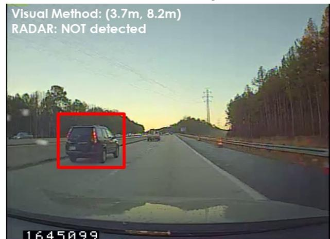
**Figure 5** Top: Radar doesn't detect the vehicle on the adjacent left lane @ FR-24609. Bottom: The same target vehicle at a later frame (@ FR-24622) is still not detected by radar as indicated by red boundary box.
