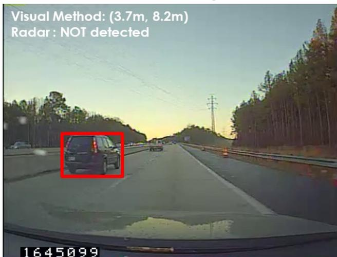
**Figure 6** Inconsistency in radar detection: Top frame shows radar detected a vehicle 5.2m away but bottom frame shows radar was unable to detect a vehicle further away
