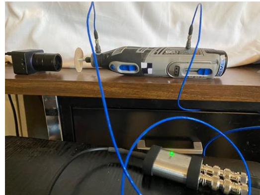
Figure 2 Cutter with accelerometers attached to signal conditioner. The event camera is shown on the bench to the left of the cutter wheel, which also has a corner target mounted on the cutting wheel. In the first experiment, we used the IMU of the event camera to estimate the cutter speed.
