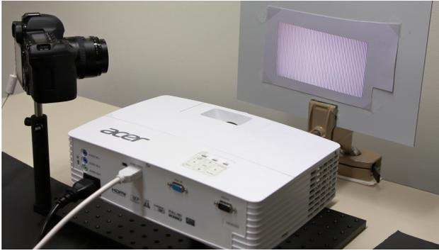
Figure 2: Our simple structured light scanner used in the experiments. It is composed of a projector-camera pair, and a flat articulated stage where the samples are placed. A sinusoidal encoding pattern is being projected onto the measured fabric.
