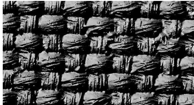
Figure 1: An image of the surface of Canon IJM 618, a coated polyester textile used as a print media. We are interested in measuring the surface roughness of printing textiles, where the weave threads form macroscopic structures.
