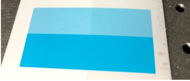
Figure 3. Picture of a glossy photoquality paper printed with two colored bands, the top one being a half-tone color of cyan ink with coverage 50%, the second one being a fulltone of same cyan ink. Half of the sample, on the right, is covered with a clear adhesive tape.
