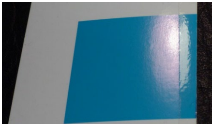
Figure 5. Photo quality paper printed with cyan ink, full coverage, partially covered by a clear adhesive polymer film (on the far right). The differences perceptible between the uncovered and covered areas are mainly due to the light reflected by the interface with air, which produces a colored pink sheen in uncovered areas, and an achromatic gloss in covered areas [5].
