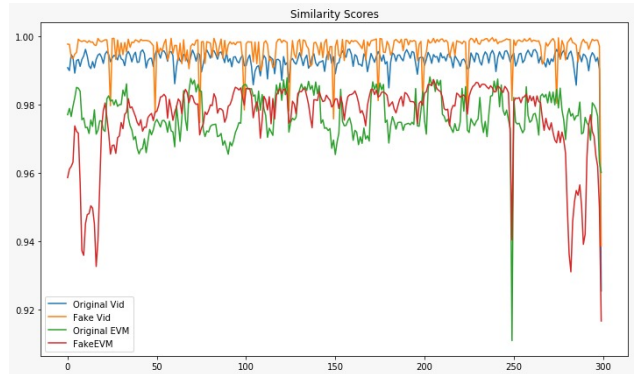
Figure 3. Inter-frame dissimilarity for original, deepfake, Euler magnified original and Euler magnified deepfake videos.
