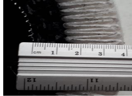
Figure 2: Cut through the filter: The thickness of the 6 different layers of the studied Filter amounts to 40 mm.
