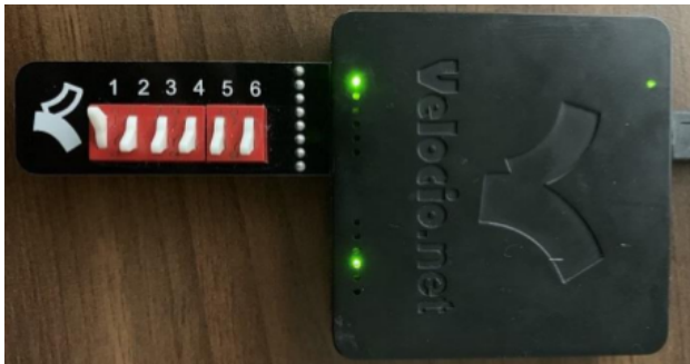
Figure 13. Correct setup of the Velocio PLC (Source: own screenshot)
