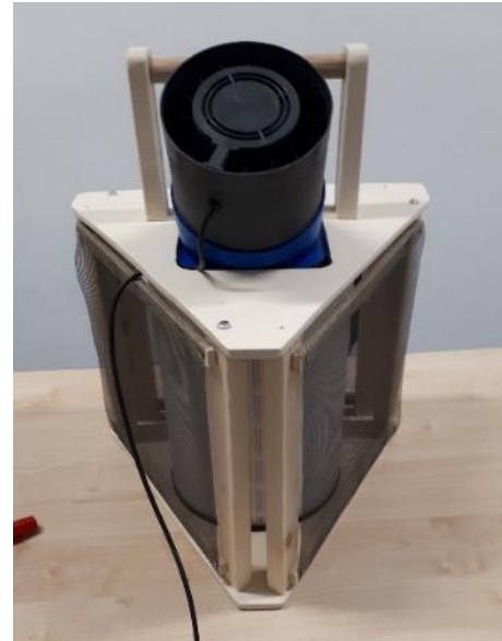
Figure 11: Purifier frame holding the filter and the 44 W fan blower. The fan's cross section of 0,0123 \text{ m}^2 and wind speed 9 \text{ m/sec} results in a flow rate of
