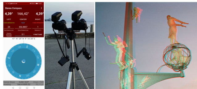
Figure 8. Bjorn Sommer presented his new StereoCompass app which can be used to plan and document stereo camera settings: Left: StereoCompass app, Centre: Two analogue SLR cameras on a tripod; Right: Red-Cyan photo of the Magic Column of Peter Lenk in Meersburg.
