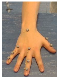
Figure 2. Preparation of hands for data acquisition with the optical tracking system QualiSys.
