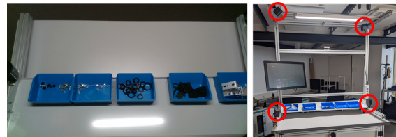
Figure 4. Left image: Camera view on the workplace. Right image: Workplace with VIVE base stations.
