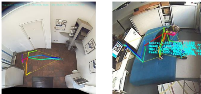
Figure 2. False detection by patterns of a ghost (left), partly false detection of the pose (right)
