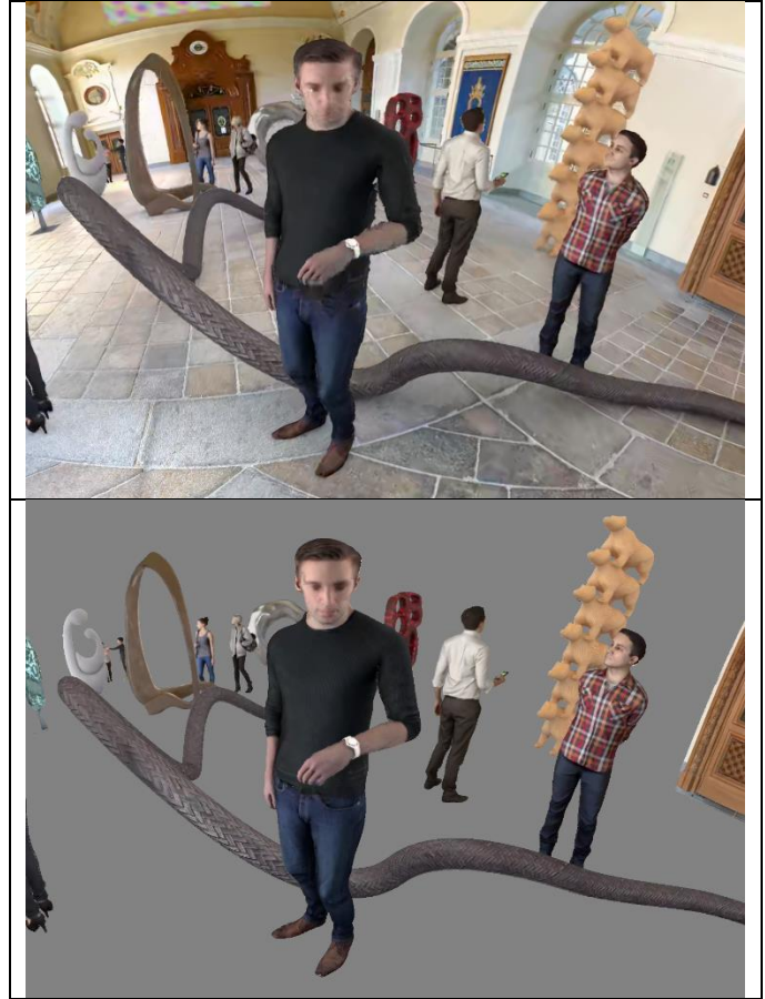
Figure 9. Subjective results of object-based solution compared to MIV anchors showing a zoomed version of v5-frame 2 of MIV anchor-QP5 (top) and object-based coding -QP3 (below). Note the subjective results are shown for different QPs but with nearly matched bitrate.
