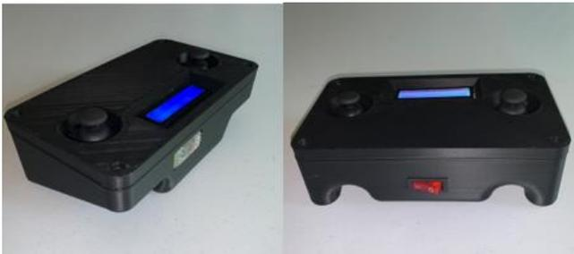
Figure 12: Printed and assembled user-input controller.
