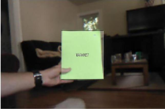
**Figure 19:** Image output from PixyMon2 software with tracking enabled. The signature box is labeled "TARGET."
