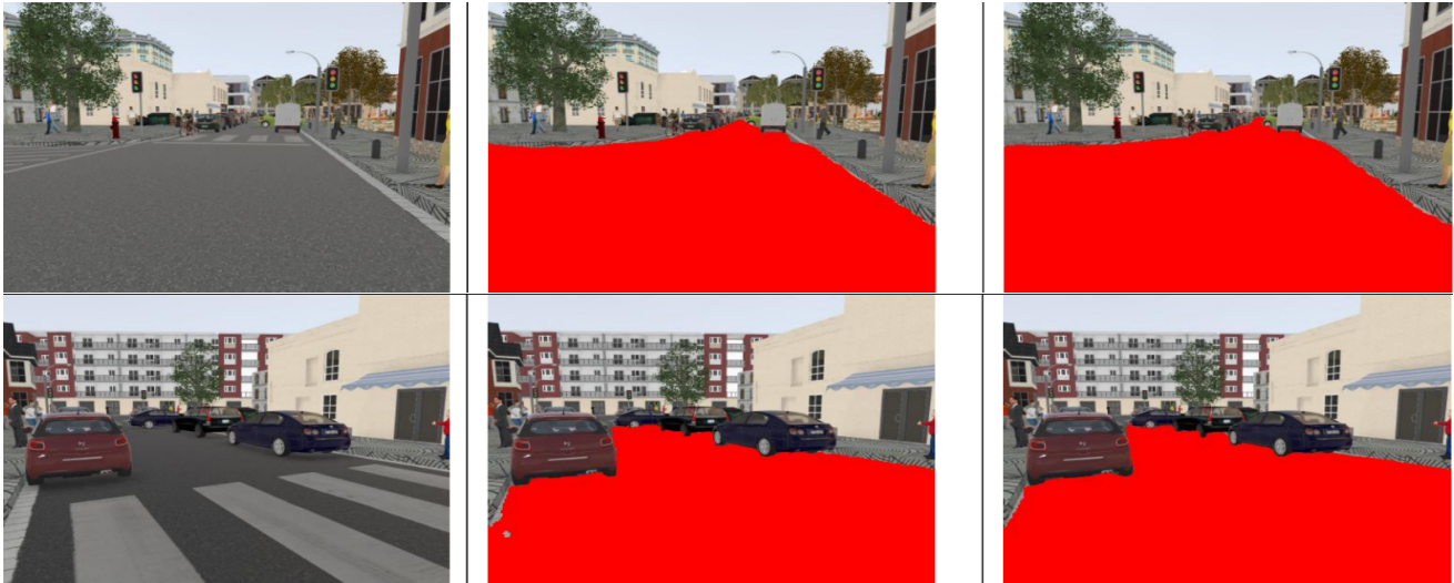
Figure 7: Semantic Segmentation Results on SYNTHIA Dataset. Original Image (left), Enet (middle) and RoadEdgeNet (right).
