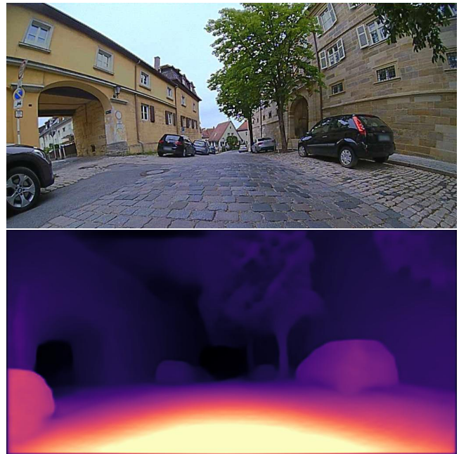
Figure 1: Distance estimation on a single fisheye image. Our self-supervised model, FisheyeDistanceNet++ , generates superior quality distance maps.
