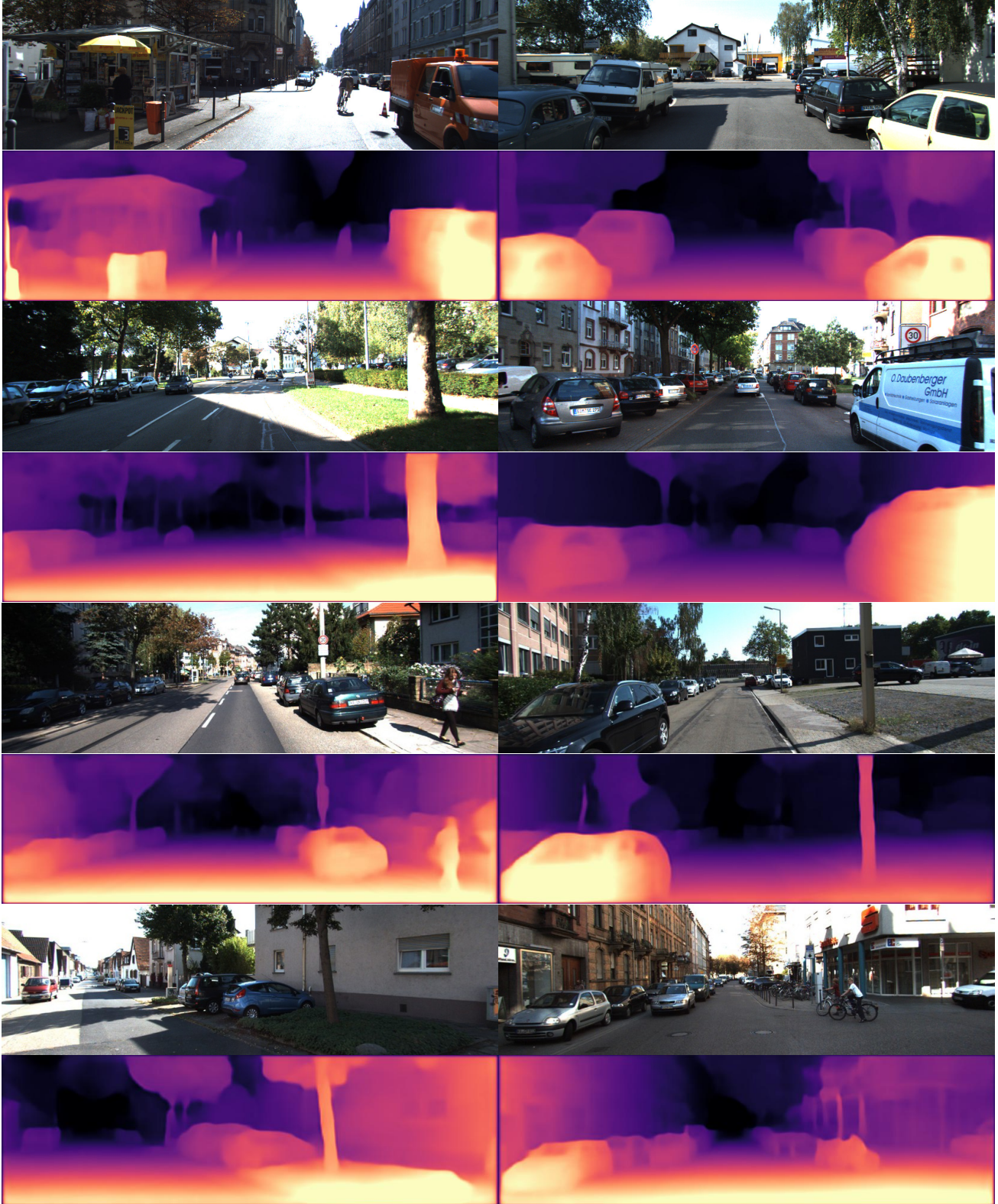
Figure 5 Qualitative results on the KITTI dataset. Our model resolves the low textured areas such as sky i.e. infinite depth and provides sharper transition in the boundaries of objects.
