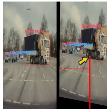
Figure 10. (left image) Truck as seen by the ego-vehicle front camera (ground truth). The Truck shown is in the driving path of the ego-vehicle. (Right image) a wrong camera calibration is applied which is still potentially seen as "successful" by the system itself. This could lead to an emergency braking event triggered too late where an accident cannot be prevented.
