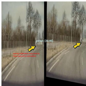
Figure 13. (left image) Pedestrian detected by the ego-vehicle front camera (ground truth). (Right image) A wrong camera calibration is applied (yaw and roll angle) which is still seen as "successful" by the system. The pedestrian is not detected by the miscalibrated device. Even if detected - the trajectory itself could be estimated and forecasted such that a possible collision is detected too late.
