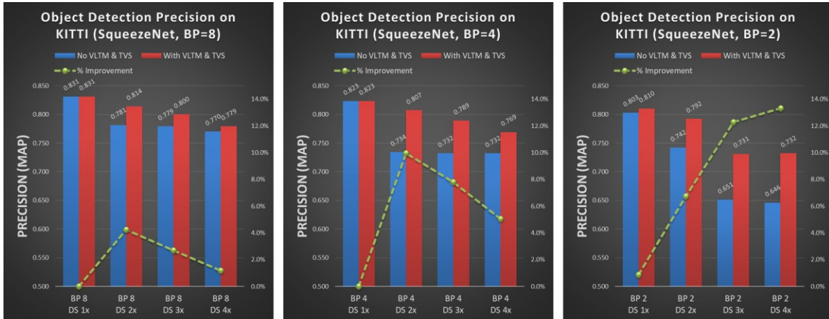
a) mAP for SqueezeNet with SqueezeDet head on KITTI data set
