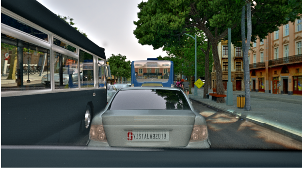
Figure 4. OI of a scene including our ego vehicle model. A part of the stray light cover as well as some distortions caused by the windshield are visible in the lower periphery of the image.
