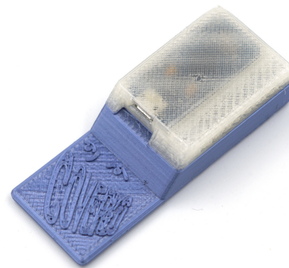
Figure 8. AMG8833-based thermal imager in 3D-printed mount
