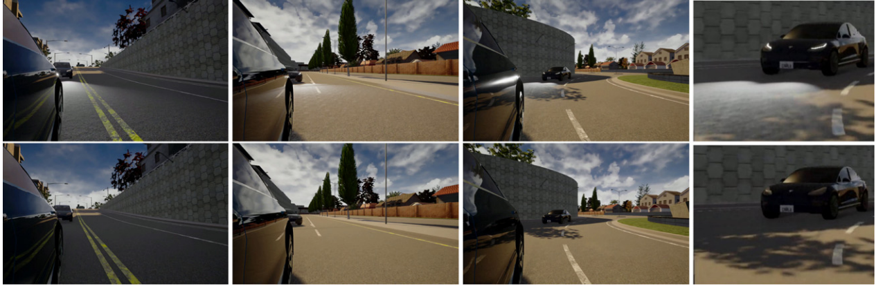
Figure 4. Synthetic capture of the left side-view mirror in chronological order of the test sequence. Captures with the following car's day running light switched on are shown at the top, and switched off at the bottom. The scene starts on a ramp (left), afterward the car turns around a corner (middle) and finally go straight through a roundabout (right). The rightmost column shows a closeup of the car's day running light, depicted from the frame shown in the third column.
