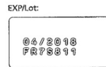
Figure 8. Binarization result obtained for images from the medicine packages used in experiments shown in Figure 5 for our novel method with haze-removal algorithm (inverted image to improve visibility).
