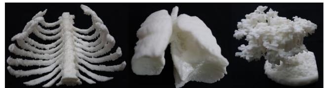
Figure 9. Physical models produced by layered manufacturing.
