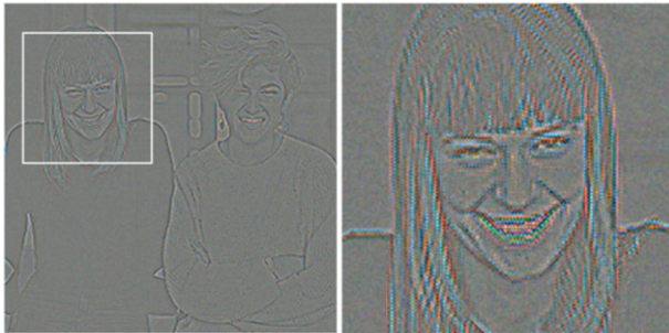
Figure 4. Artifacts of fixed pattern caused by demosaicing the Branca et al. [18] “People” image (left) and the detail of it (right); image contrast was enhanced.
