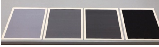
Figure 3. Print samples with tint levels 30%, 50%, 70%, and 100% were printed with a prototype large-format printer using a page-wide array inkjet print bar. We selected 12 samples from levels 30%, 50% and 70%, and 6 samples from level 100%, resulting in a total of 42 test samples.
