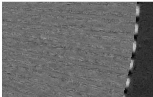
Figure 9. Noise-only image near the edge of star for camera 2 JPEG at ISO 25600.
