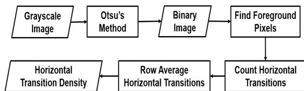
Figure 7: Workflow for calculating horizontal transitions. Calculation of vertical transitions proceeds in a similar manner.
