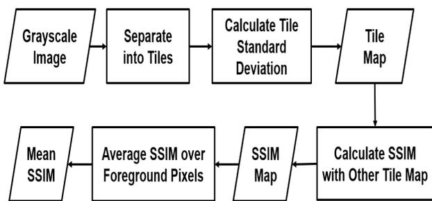
Figure 4: Tile-SSIM workflow.
