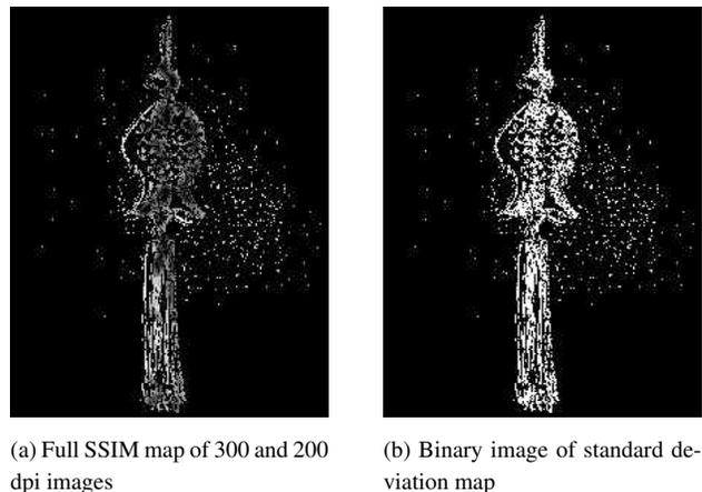
Figure 5: Full SSIM map and the binary image of the standard deviation map. From (a) and (b) we can tell that the binary map provides a good mask to locate foreground pixels, so that background pixels will not affect the quality assessment.
