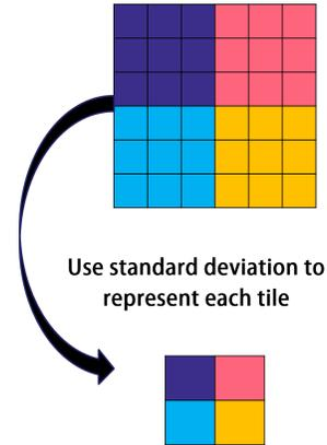
Figure 2: Steps to generate standard deviation map. The above block shows the original image and the tile size of  $3 \times 3$ . After calculating the standard deviation of each tile, we form a new standard deviation map, which has the same size across all resolutions.
