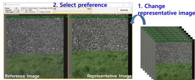
Figure 3. GUI of the pair-wise comparison based subjective image quality assessment. A left image in main GUI is reference and a right image is representative test image.
