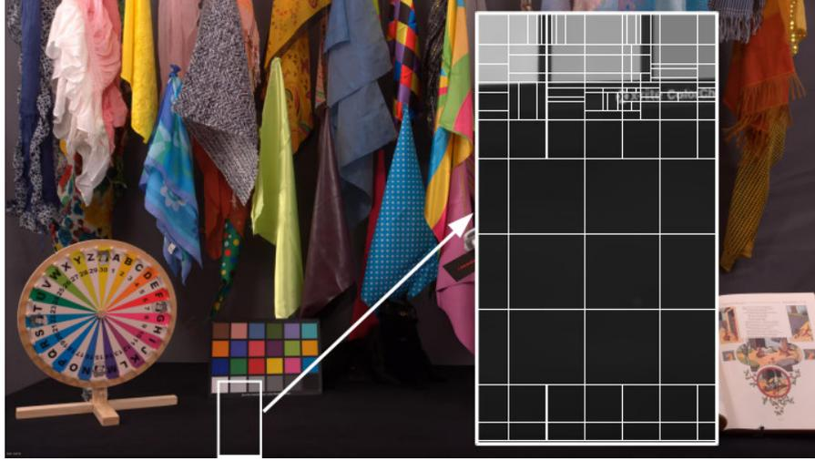
Figure 2: Example of CU structure partition of the VTM3.0 for sequence CatRobot (3840 × 2160).
