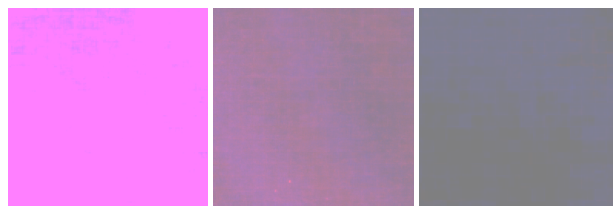
Figure 14. Color noise for each pixel of a 18% gray patch for Huawei P20 at 1, 100, and 1000 lux
