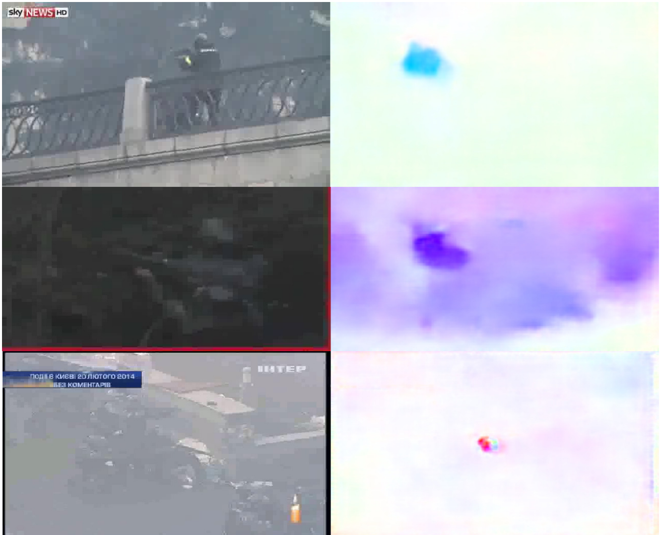
Figure 12. Comparison between original video frame and its respective Optical Flow graph. Left: Video keyframe with Visible Shooting. Right: Optical Flow Graph showing clearly the shooting smoke.
