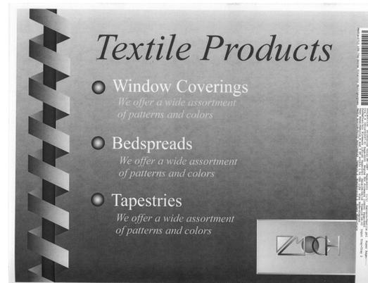
Figure 1. A printed image with mottle defect.
