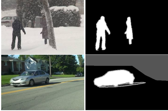
Figure 4. Sample images from the Change Detection 2014 dataset [15]. The left column contains sample images, while the right column consists of pixel level ground truth.
