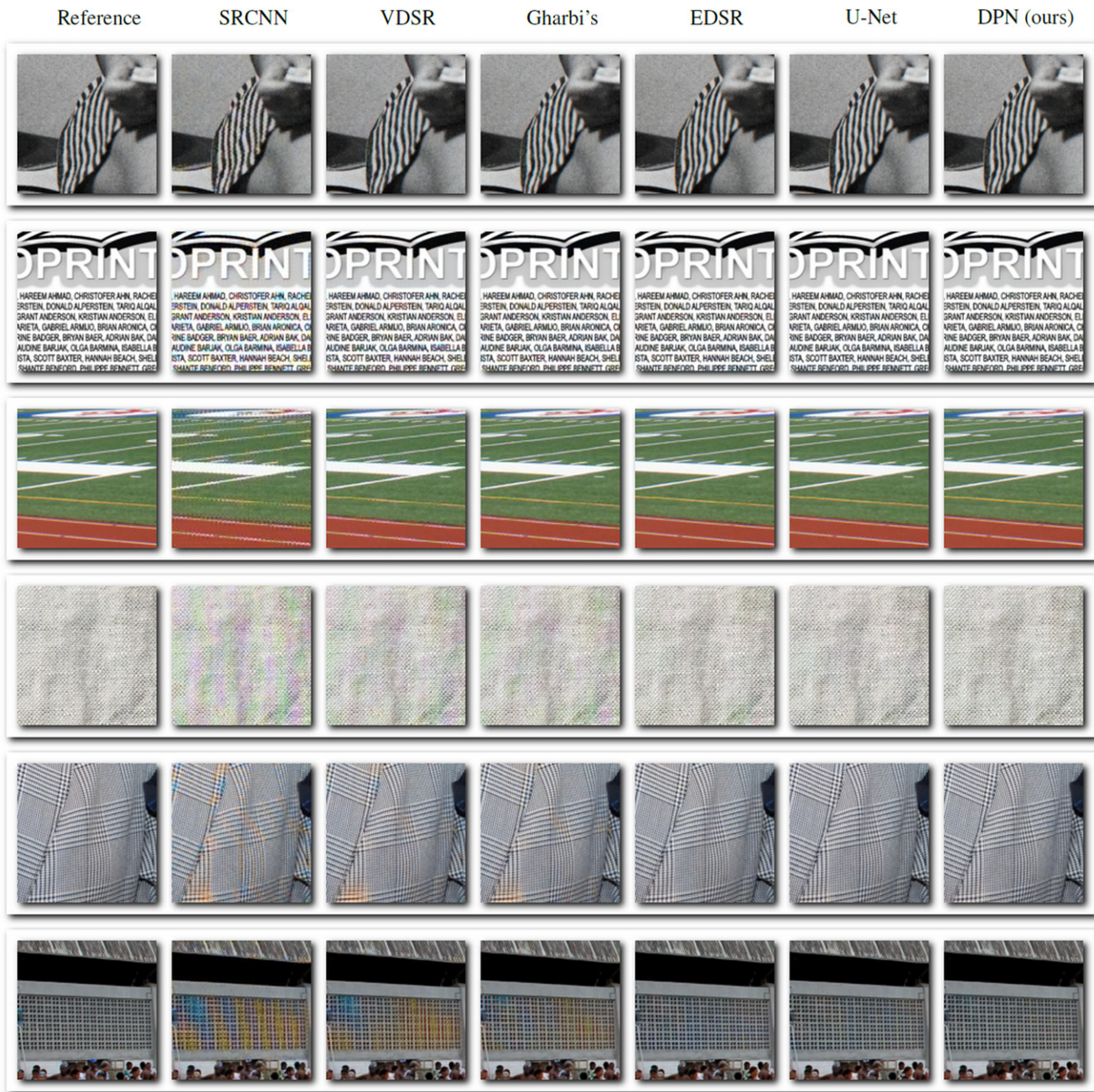
Figure 13. Image quality evaluation results on Moire dataset [8]: improved color moire and false colors versus state-of-the-art (images 19, 158, 166, 182, 209, 334).
