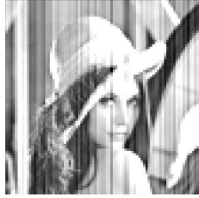
Figure 10. Columnar Fixed Pattern Noise generated by the simulator
