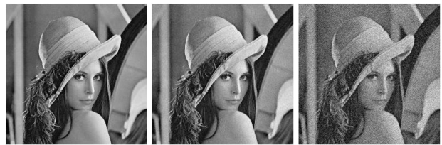
Figure 9. Variable readout noise. Readout = 0, 50, 200 e-. Maximum number of photons received by one pixel = 6000. Full well = 7000 e-.
