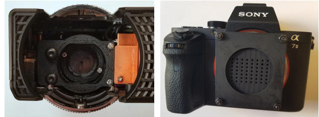
Figure 8. Projector lens (left) have been modified to obtain small, closely focused image and to include a small aperture. A full-frame camera (right) has a custom lens array system installed comprising of a pair of lens arrays (to decrease the focal length) and apertures array is between.
