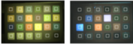
Figure 2. Raw camera images captured when the MCC is illuminated with the broadband “white” LEDs (shown on the left), and short wavelength “blue” LEDs (shown on the right). The rectangles superimposed on the images indicate the image area over which the mean R, G and B pixel responses were calculated. Many of the patches include fluorescent pigments that are visible when illuminated by the “blue” light. The fluorescence will also be present when illuminated by the “white” LED light, but the number of fluorescent photons is very low compared to the number of reflected photons.
