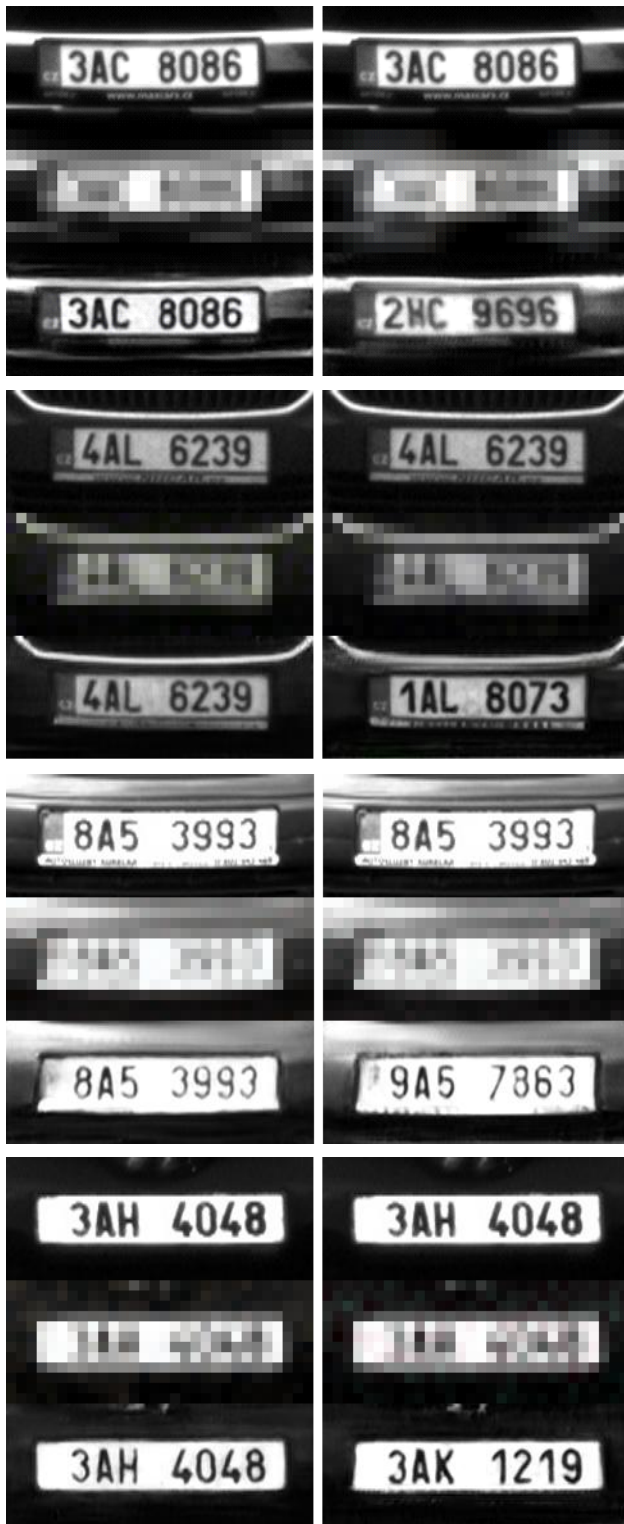
Figure 2. Four examples of the outputs of our network on the left side of the pairs of the images and the outputs of pure GAN on the right side. First rows are original images, second rows show up-sampled noisy low-resolution images and the last rows present the outputs.
