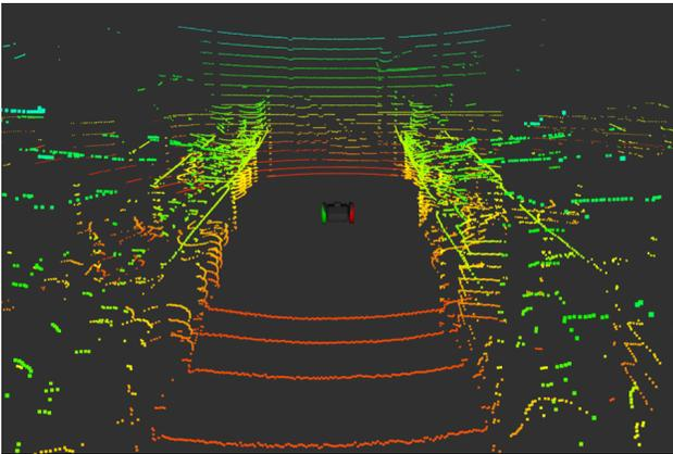
**Figure 3.** Point cloud visualization of Velodyne VLP-16 3D LiDAR readings inside the warehouse testing environment. The agent is in the same location shown in the omnidirectional image from Figure 2.
