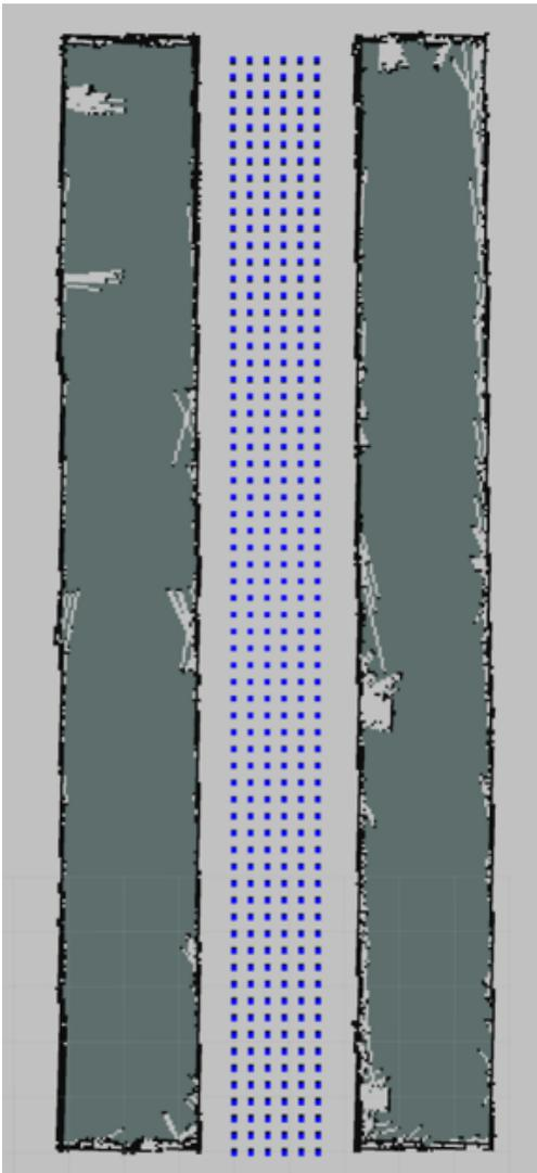
**Figure 6.** Coordinate layout of localization evaluation environment. Six horizontally spanning intersection points are positioned 0.3048 meters apart. The vertically spanning intersection points are spaced 1.828 meters apart. An additional buffer region is placed between the recorded coordinates and the aisle shelves.
