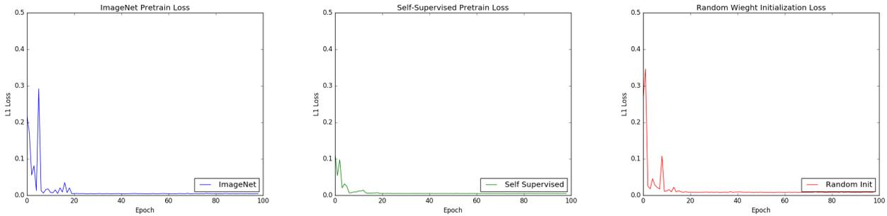
**Figure 7.** Omnidirectional camera localization model validation dataset loss during training for the ImageNet (left), four patch self-supervised (center), and random initialized (right) networks. A learning rate decrease occurred every 20 epochs. Convergence speed and overall loss stability is greater for the self-supervised pre-trained network compared to the ImageNet and random initialized networks.
