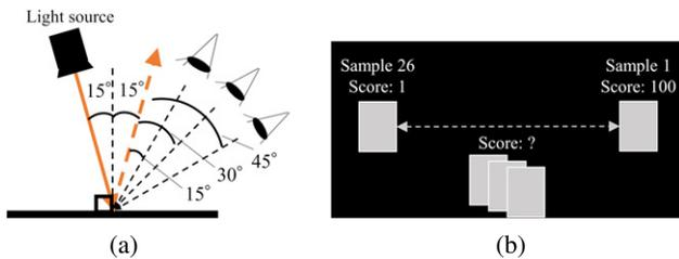
Figure 10. Subjective evaluation experiment: (a) experimental conditions and (b) experimental procedure.
