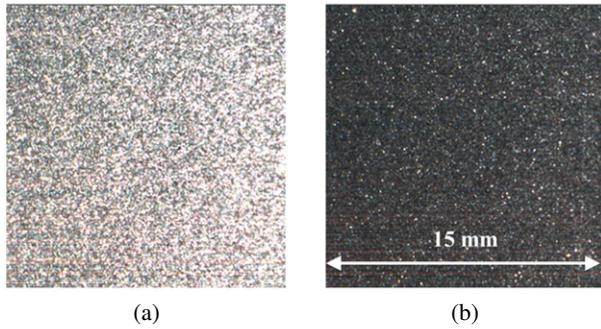
Figure 1. Example of the sparkle impression: (a) surface observed from the highlight angle (near the specular condition) and (b) surface observed from the shade angle (diffuse reflection direction).
