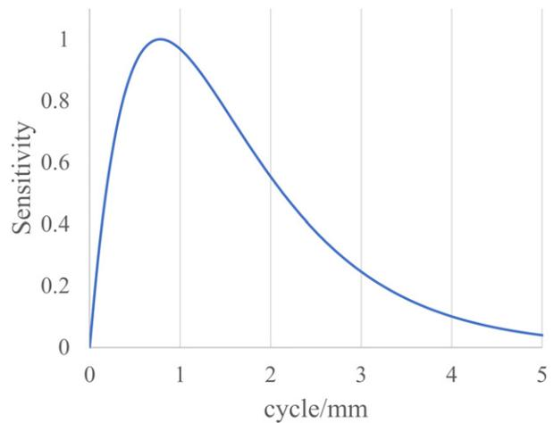
Figure 8. Human visual characteristics for an observation distance of 400 mm.
