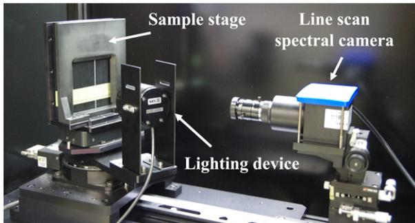
Figure 3. Measurement device.
