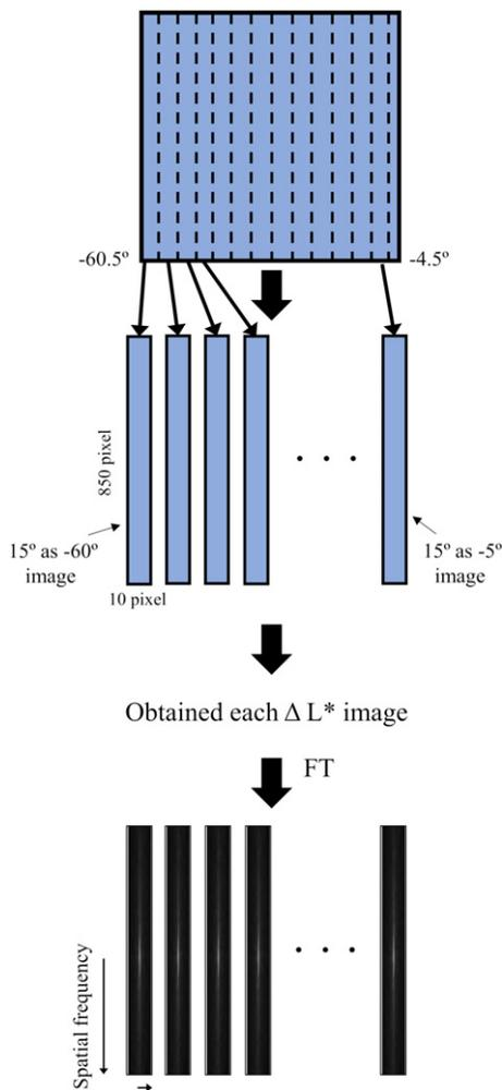
Figure 7. Procedure of calculating the spatial frequency characteristics every 1° from the  $L^*$  image.
