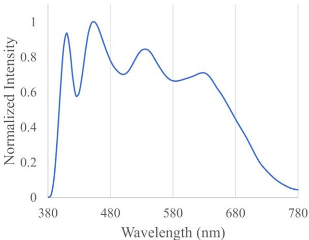
Figure 4. Spectral characteristics of the natural-light LED illumination.
