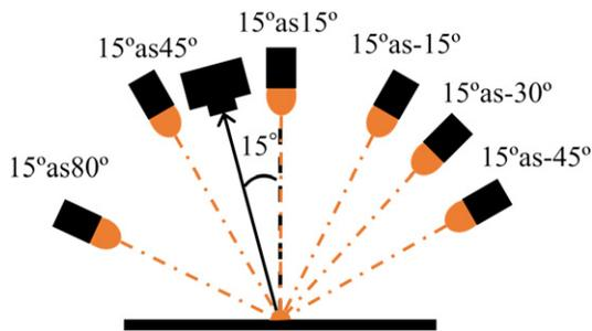
Figure 12. Measurement geometry of the MA-T12.
