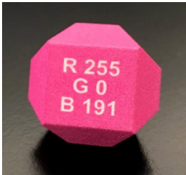
Figure 6: Color values communicating the sRGB values that should be used for 3D objects to achieve the corresponding 3D printed color.
