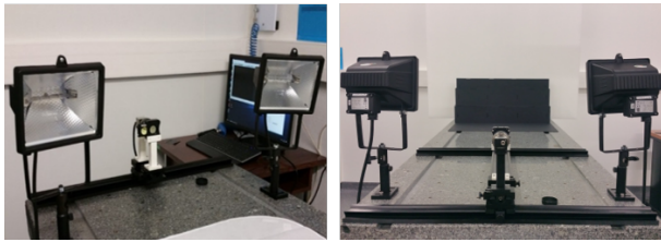
Figure 2: Overall view of our multispectral image acquisition bench: sensor and light sources (left), scene seen from sensor point of view (right)
