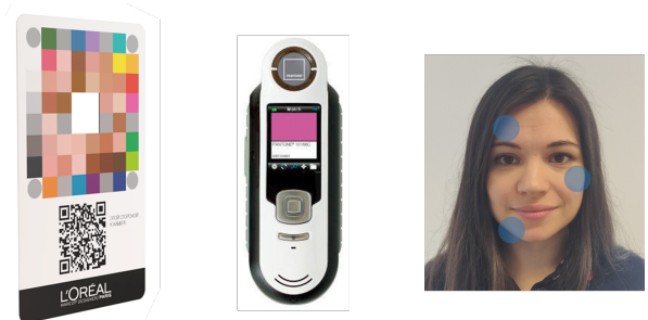
Figure 3: Left, an Xrite CapsureMe used as a color calibration target in our study. Middle, a Xrite Capsure, the spectrophotometer used for measuring panelists skin color. Right, the position of the three measurements on the face
