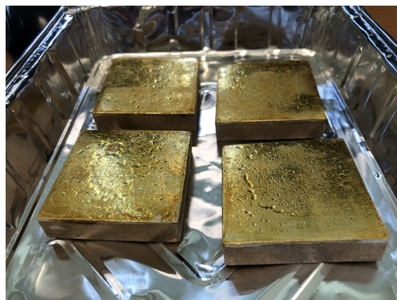
Figure 2. Condensation on the surface of four mock-ups after freezing.
