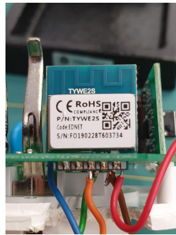
Figure 6. Microcontroller with Soldered Extensions
