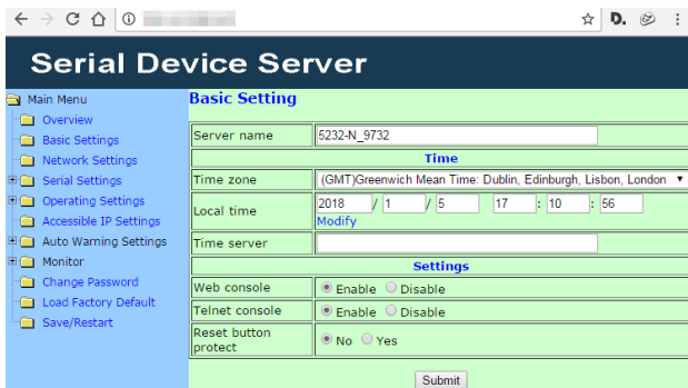
Figure 18. Web interface of a Moxa 5232-N (found in Shodan January 2018)
