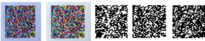
Figure 5. Example of JAB code printed by an unaligned Inkjet printer.
