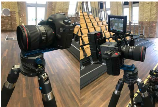
Figure 21. Placement of DSLR camera (left) and movie camera (right) on panorama head
