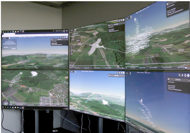
Figure 8. The Tiled Stereoscopic 3D Display Wall showing different perspectives of a bird flock trajectory data set.
