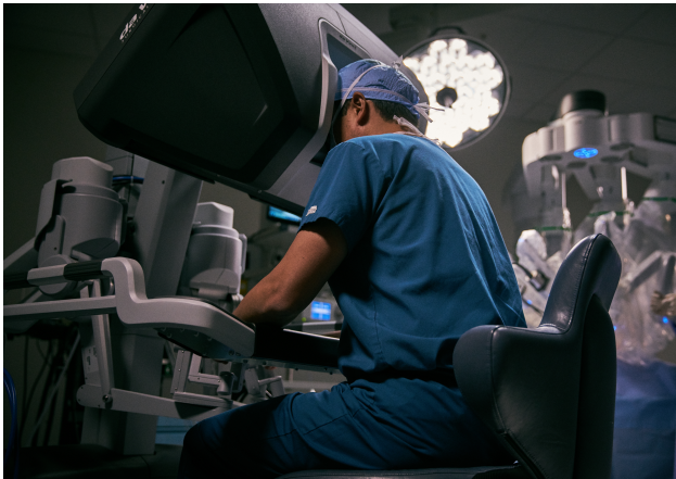
Figure 12. Da Vinci X surgical system from Intuitive Surgical enabling stereoscopic distant surgeries. (Courtesy of ©2020 Intuitive Surgical, Inc. All Rights Reserved.)
