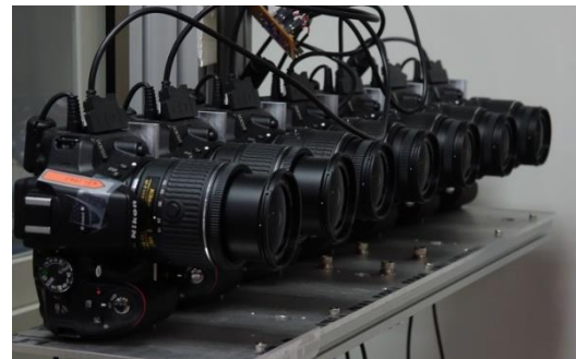
Figure 1. The proposed camera array system consists of 7 DSLR cameras and one external triggering circuit, that are connected with a computer.
