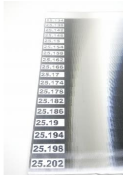
Figure 6. Black-white stripes printed with several lpi are used to verify the proper printing resolution
