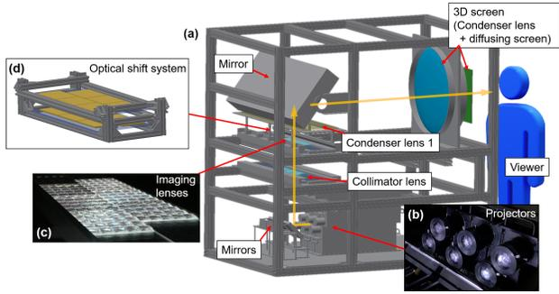
**Figure 7.** Developed display system: (a) overall view in the system, (b) six projectors, (c) imaging lenses arranged in two-dimensional array, and (d) optical shift system used for TDLS experiment.
