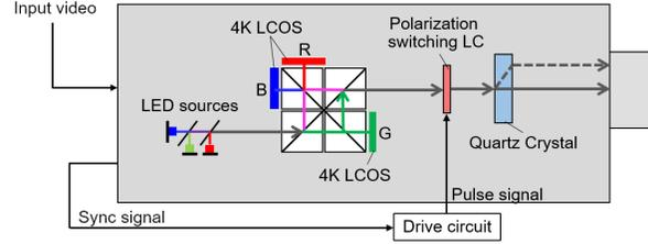
Figure 3. Developed 4K Projector with wobbling device.
