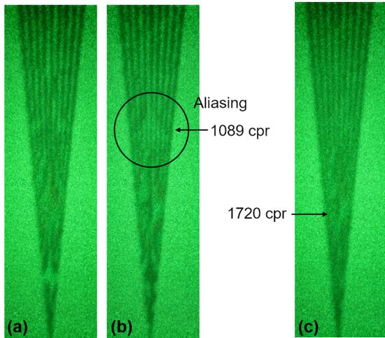
**Figure 9.** Results of 3D images displayed at 20 mm of depth from the screen to front side of (a) odd frames and (b) even frames without Wobbling, and (c) with Wobbling.
