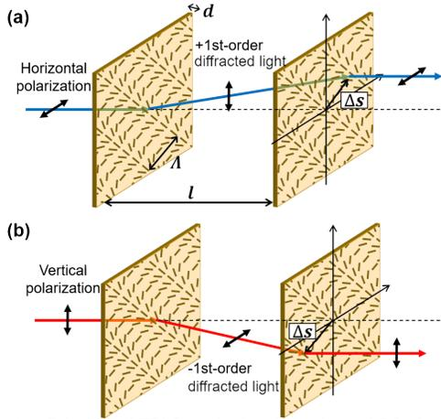
**Figure 4.** Principle of TDLS method and functions of PGs in the case of input incident light of (a) horizontal polarization and (b) vertical polarization.
