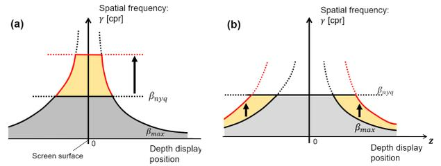
**Figure 6.** Resolution characteristics of 3D image in (a) half of pixel pitch with wobbling and (b) half of viewpoint interval with TDLS.
