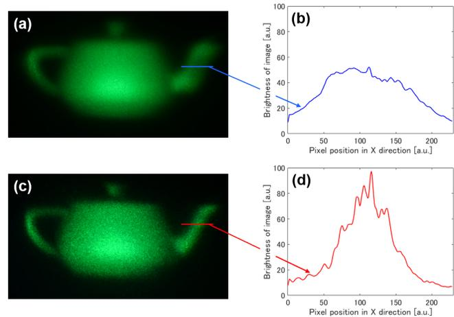
**Figure 10.** Results of 3D images displayed at 100 mm of depth from the screen to front side and brightness profiles of 3D images: (a) and (b) are results without TDLS, and (c) and (d) are results with TDLS.
